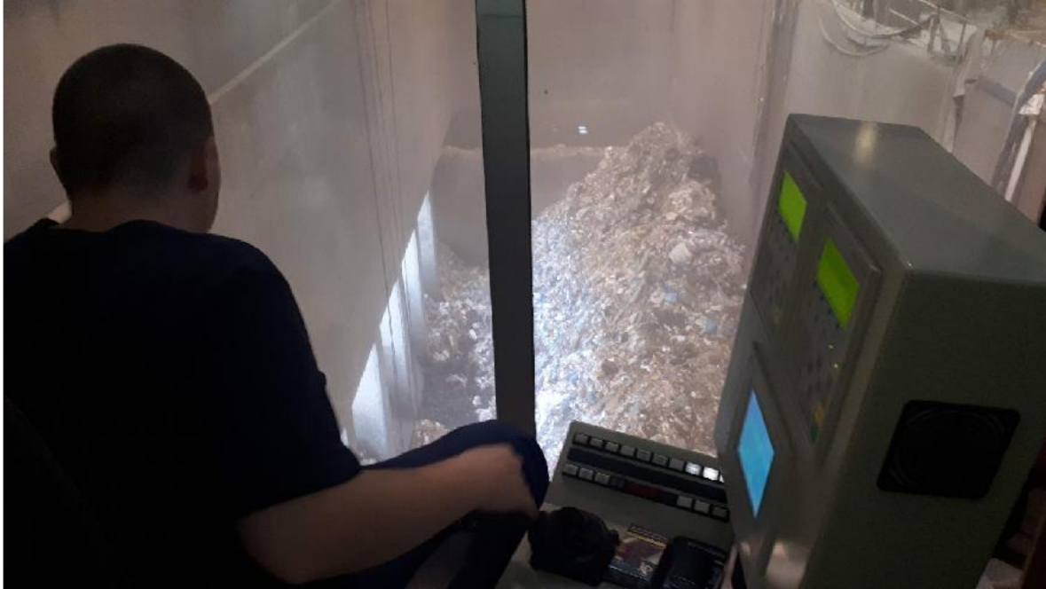
Crane being used to move mixed garbage to incinerator
